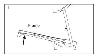
Hold the treadmill firmly with your right hand as shown. Pull the latch knob to the left and hold it.
